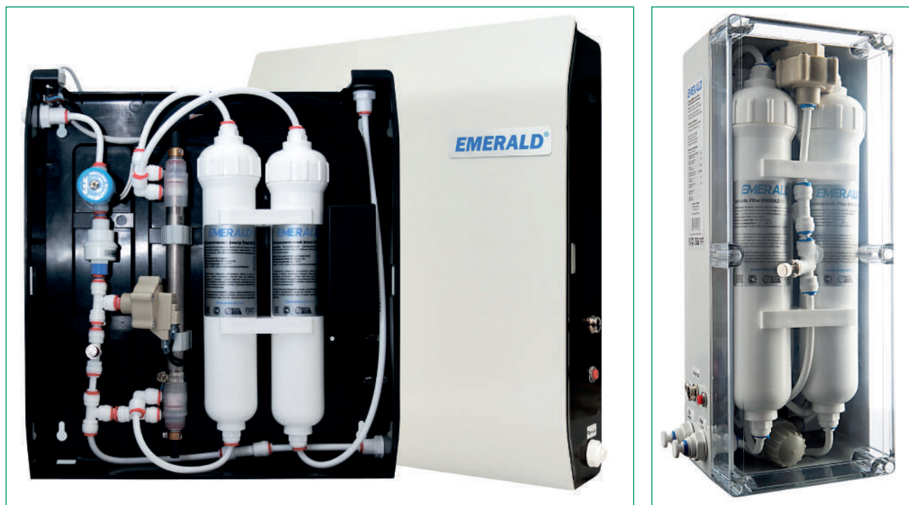
Fig. 6.2.4. EMERALD HOME devices based on MB-11 elements of the latest generation, manufactured under license by EMERALD ECOTECHNOLOGIES LLC. EMERALD devices of HOME series are used in flats, offices, cottages and various public places, providing the best achieved degree of water purification and conditioning. On the left is EMERALD HOME 40 device, productivity — 40 l/h, power consumption — no more than 30 W, 2018. On the right is EMERALD HOME 60 device, productivity — 60 l/h, power consumption — no more than 60 W, 2019.
