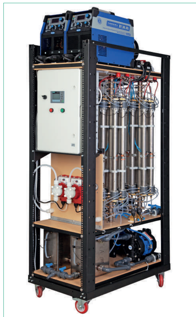
Fig. 6.2.6. AQUATRON-15-1500E device. The reactor of the device is made of twelve flow-through electrochemical modular elements MB-26T of a new generation with the use of ultrafiltration diaphragms made of chemically pure alumina in the alpha form.
